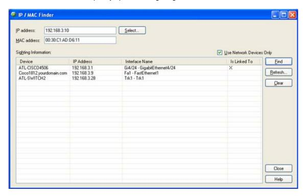
When enough network data is available, IP/MAC Finder indicates to which network interface the IP or MAC address is physically connected.
