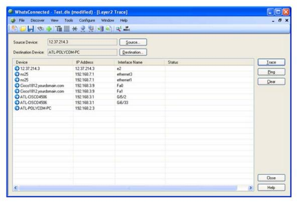
Using previously discovered network connectivity data, the Layer 2 Trace tool finds the path between the two devices and then displays each network interface that is used to build the path. The trace tool also allows for a quick check of the status and availability of each step along the layer 2 path.
