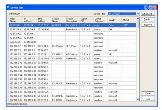
You can filter data displayed in the view by using the Device Filter and Advanced features.
