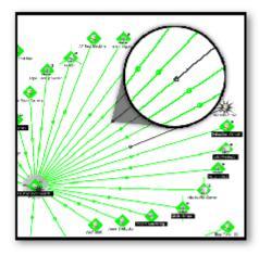
In the graphic above, there are two link lines connected by a dot in the center of the line between the two devices. This shows that the devices are linked in both directions. This is done by repeating the process above from the second device, back to the first. Now, when one of the links goes down, you can see on which side the problem occurs.
