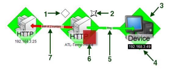
**Passive monitor indicator**. A diamond shape at the upper left of the device icon, displays the state of the passive monitors associated with the device.
