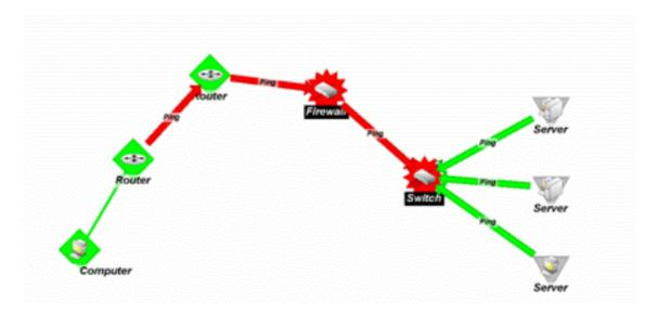
Down dependencies are useful in showing the break position in a chain of machines. If the chain is not broken at any point, the machines in the chain are not polled and are assumed up.
