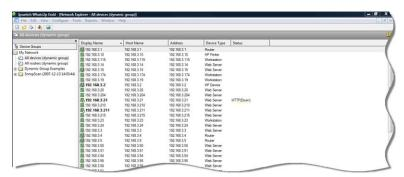
Each device's icon provides information about its device state and the state of the monitors associated to that device. In addition, the Status column indicates which specific monitor is down and the duration of the interruption.
