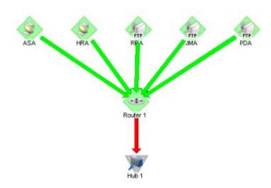
In the example above, the devices have an up dependency on the router, and the router has a down dependency on the hub. If the router's active monitors fail, the hub would be polled, and the devices behind the router would not be polled. When the router's active monitors are successful, the hub is not polled, but the devices behind the router are.
