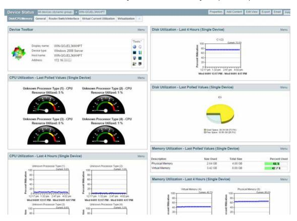
Throughout the web interface you will see links to devices, such as HP ProCurve Switch. All of these links point to the Device Status dashboard for that device. If there is a potential problem with a monitored device, the Device Status dashboard is a good place to look for more information about the device status.
