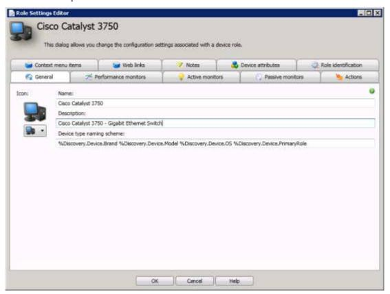
WhatsUp Gold provides several default device roles that are used to identify most common network devices. These default roles should correctly identify the majority of devices on the network, but you can modify the device roles to customize what is monitored on each device and what action policy is applied. Device Roles are managed in the WhatsUp Gold console (File > Discover Devices > Advanced > Device role settings).
